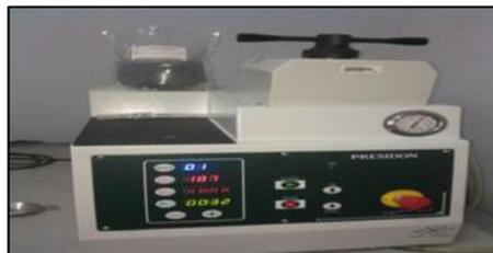
Gambar. 3.9. Mesin *Mounting*
